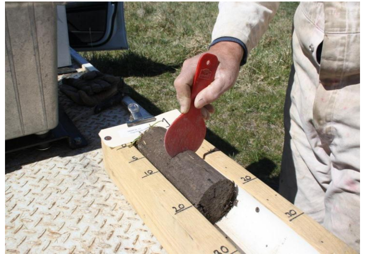
Cutting up Soil Core to measure bulk density of the soil
