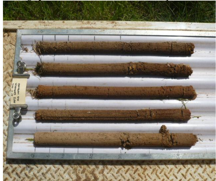
Soil cores to 50cm, collected for cutting into 10cm depths for analysis
